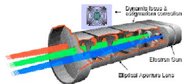
Hitachi Elliptical Aperture, Dynamic focus (A-EADF) Electron Gun
